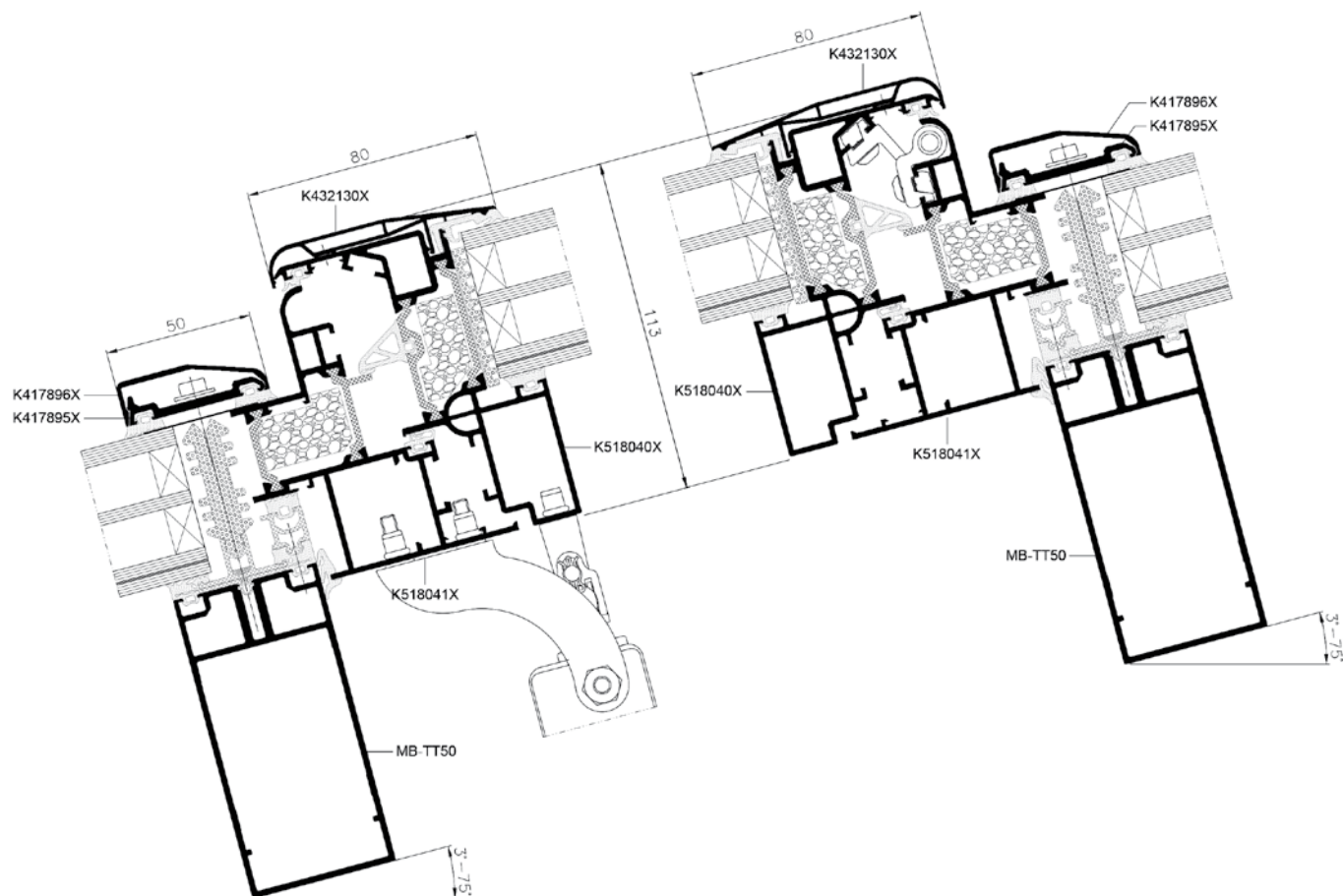
Cross-section of the the MB-70 system's smoke exhaust window
