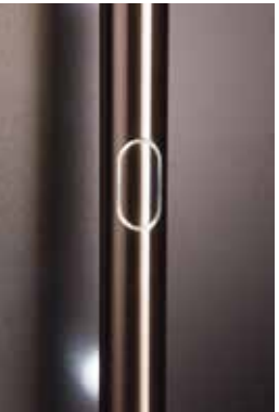
Touch sensor set into the pull*
